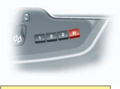
If button 1, 2 or 3 is not pressed within seven seconds of the **M** button being pressed, the memory function will cancel.
